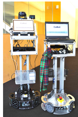
Figure 1: Our CoBot robots are capable of autonomous localization and navigation, but cannot manipulate objects.
